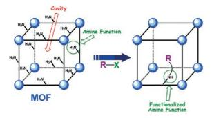
A new metal-organic framework with amino groups oriented inside the pores has been synthesized. The post-synthetic modification of the cavities in this MOF with two different functionalities is for the first time clearly evidenced by X-ray crystallography. The cavities of the MOF can be transformed without modifying the original 3D structure of the MOF.
